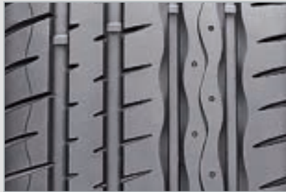
Continuous rib patterns improve longitudinal stiffness.
